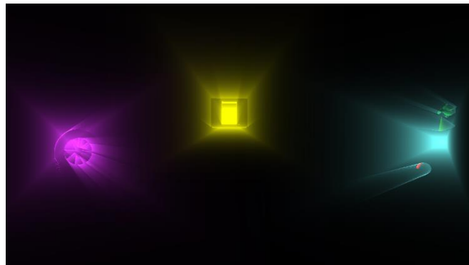
Figure 8: Main screenshot of the demo. The demo shows a scene divided into three parts: left, center and right, each part with its own light. Each light has a different intensity and color, no falloff and a 512x512 resolution shadow map.
